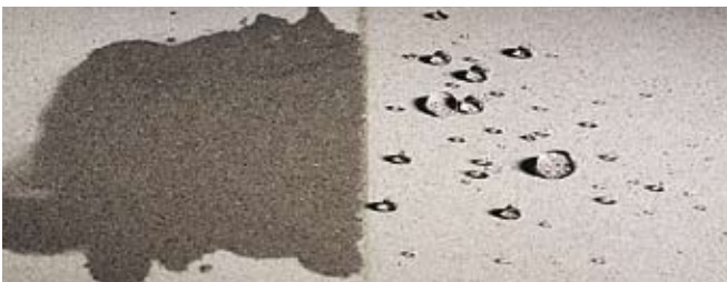
Water-repellent protectors prevent water from penetrating, creating the so-called "drop effect" clearly visible in the photo.
