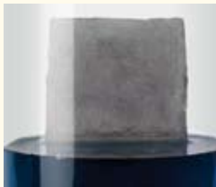
A metal edging dipped in hydrochloric acid; the aggressive effect of the acid is obvious.
