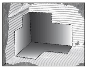
Continue with thin-set along the floor-to-wall transition from the corner outward for the first strip of HYDRO BAN Sheet Membrane Sealing Tape. Overlap the corners by 2" (50 mm).  Lay the tape and remove all air pockets and excess material as with the corner piece.
