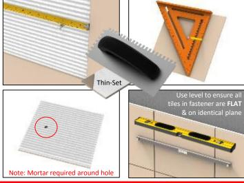
Note: System will not work on tile thicknesses less than 5/32" or greater than 1/2"
