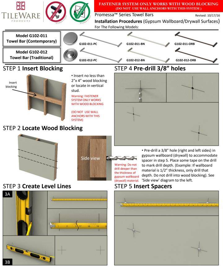
As illustrated in 3A - Use a level to determine position of right spacer and mark a vertical line. Measure precisely 18" from this line to locate the position of left spacer.
